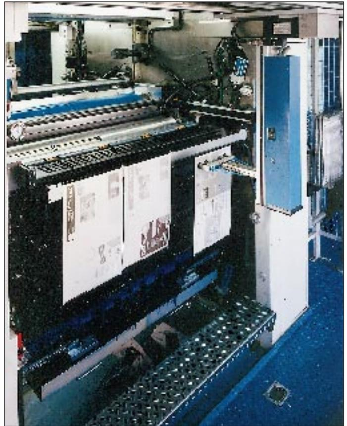
*At the four-high tower of the KBA Express newspaper rotary press, robots carry out the mounting, or changing respectively, of the plates.*
