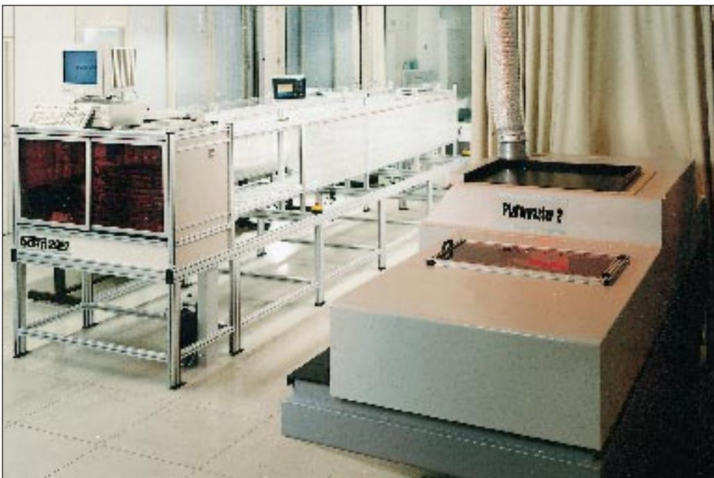
*The automatic plate sorting system (left), a development by the newspaper house, puts the press-ready plates into the transport cassettes of the conveying system in accordance with their positions on the cylinder.*
