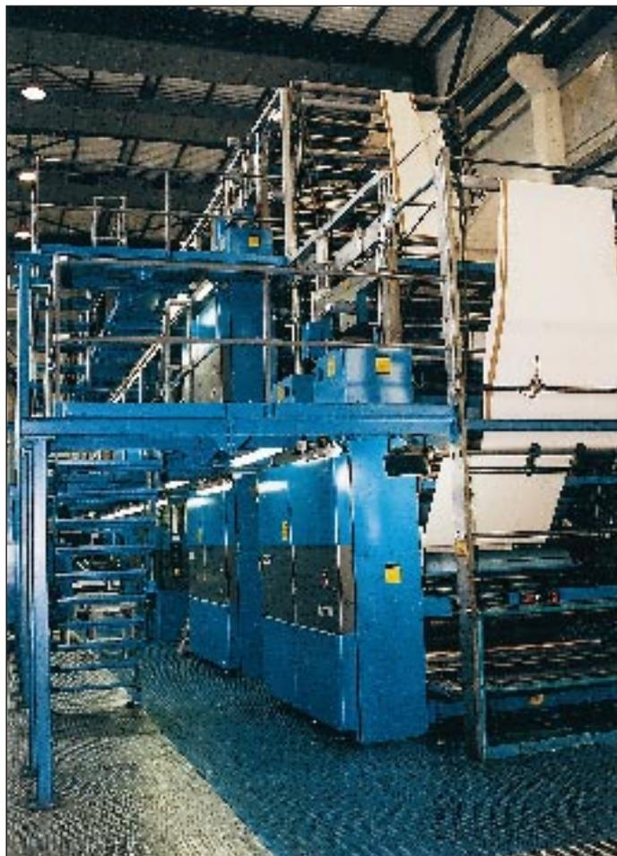
Left: El Diario de Navarra has its own radio broadcasting station. Right: The Goss HT 70 rotary press has been in operation for a little more than one year.
